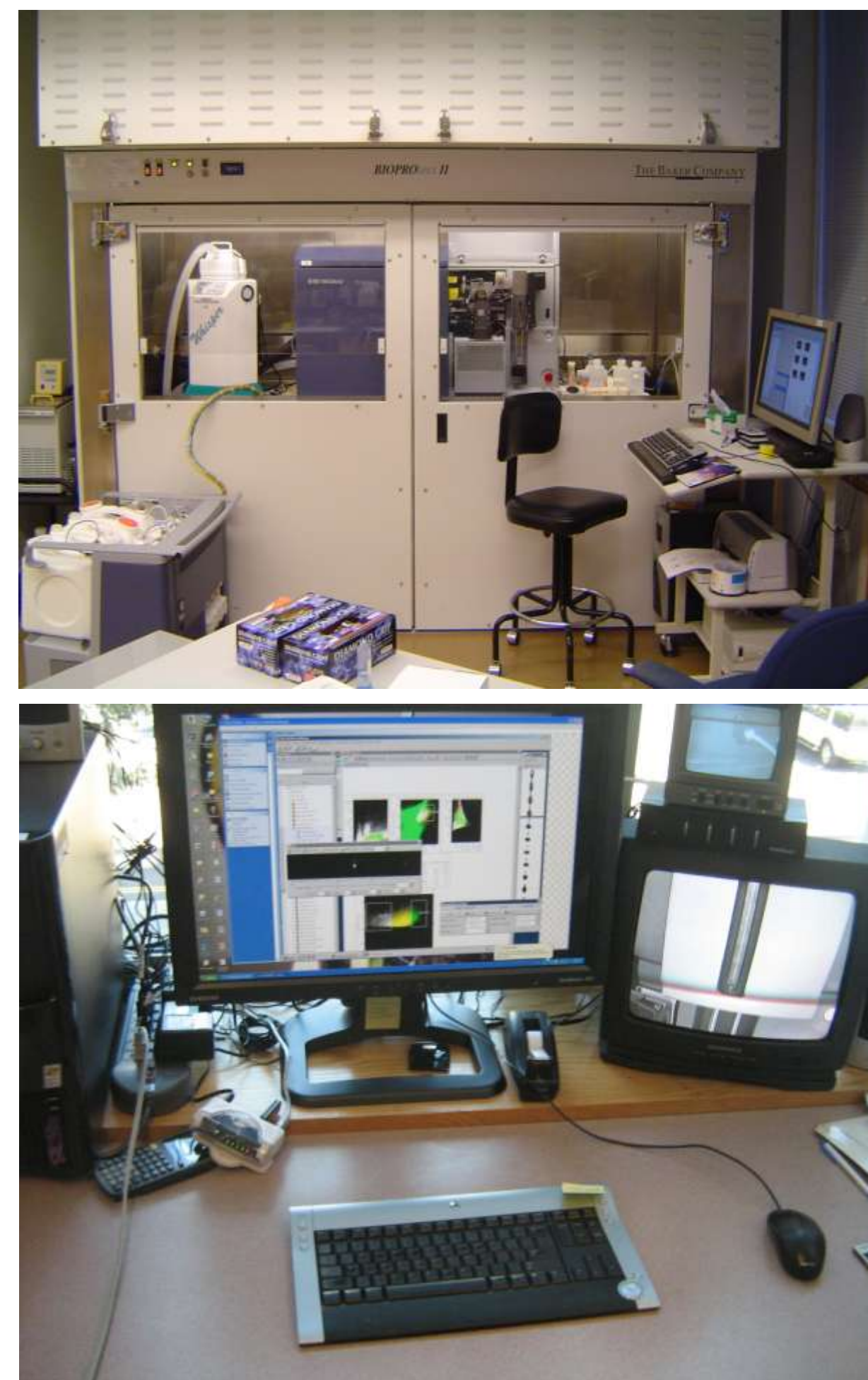
Figure 2. Biohazard sorting and analysis of cells from immunized mice using FACSria located inside a biological safety cabinet Biohood Baker II (top panel). System is equipped with an aerosol management system (BD Biosciences) and self-designed remote-control unit (bottom panel). Remote-controlled sorting approach was developed for sorting cells infected with airborne pathogens.
